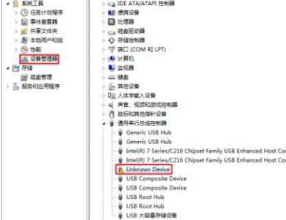
2. If the driver cannot be found in the "Device Manager" after inserting the serial cable, but it displays "Unknown Device", then change another USB port on the computer to test. If this problem still occurs, the serial cable may be faulty. It is recommended to return it to the factory for replacement.
